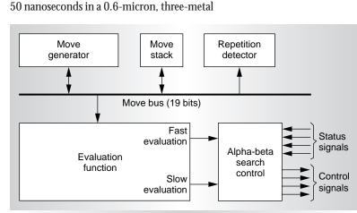
Figure 1. Block diagram of the chess chip.
