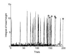
Fig. 13. Time course of learning with real robot. Circles show 10th successful stand-up, upon which a simulation run was terminated.
