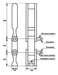
Fig. 11. Real robot configuration.
