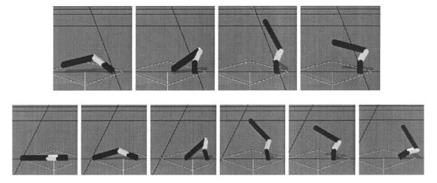
Fig. 4. Example of a sub-goal sequence after 300 trials (top); example of a failed stand-up trajectory after 300 trials (bottom).
